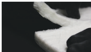
Cutting aerogel, exposed edge fraying
