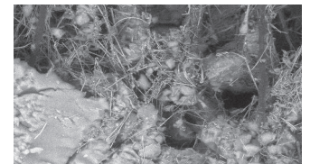
Microscopic SEM image of AlkeGel blanket showing superior interlocking qualities of aerogel particles and fiber matrix
